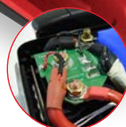
No solder high current connections
