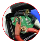
No solder high current connections
