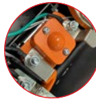
No solder high current connections
